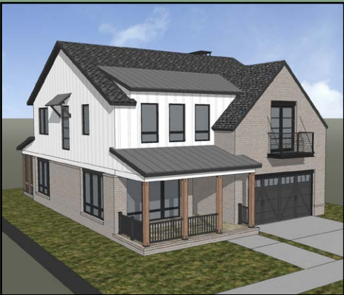
Limit garage freeboard to less than 24” using architectural elements and style-appropriate roof forms
