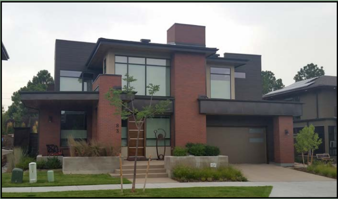
Provide garage doors with deep trim, decorative panels, windows, and other architectural embellishments to provide deep shadow lines and depth.
